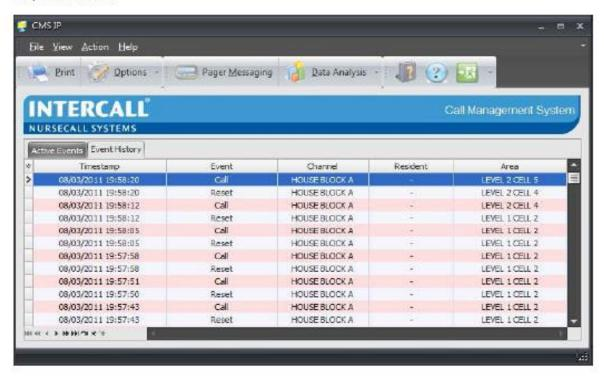
The CMS Lite software connects to the same Local Area Network as the L7700 L7700 IP Controller. With the use of an additional IP L7744 interface, free text messages may be sent to Message Pagers and DECT telephone handsets. A typical installation is shown below. The software is licensed for use on any number of computers on the same Local Area Network.
